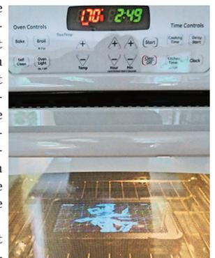
ture was an overall 208,107 CrystalMark score. At 170F, the XSLate B10 scored a 203,466. That's a full 97.8% of its room temperature benchmark score, and well within the +/- 2.5% deviation we usually see when we run the same benchmarks multiple times.
