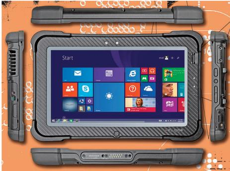
The front shows that the machine was designed to be used in landscape mode, but it quickly snaps into landscape or upside down mode if the tablet is turned. For hardware controls, there's a physical Windows button in the bottom center of the face. Above the display is the camera as well as dual microphones (the Bobcat only had one). To the right of the screen is a small indicator light that shows battery status.
