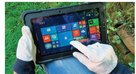
But what about "wet" touch? That's more tricky because you can't measure touch capacitance between two electrodes when it rains onto the surface. Water is an excellent conductor, and water sprayed or falling onto a touch screen makes accurately detecting capacitance between electrodes impossible. One approach, at the cost of losing multi-touch and just having touch, is self-capacitance where the capacitance between one electrode and the ground is measured.
