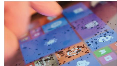
So how does Xplore's "wet" mode work? We don't think it's self capacitance. Instead, we think wet mode provides touch functionality by significantly decreasing the sensitivity of the touch controller and using a special screen protector that makes water pearl and bead enough so that there isn't uncontrolled conduction between different parts of the display surface. We could be wrong, but that's how it felt.
