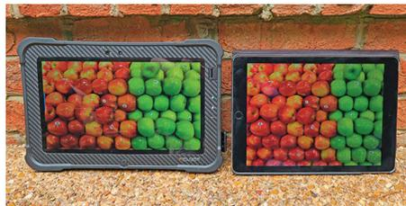
Current display technology, however, remains a compromise. Glossy screen surfaces make for a pleasant viewing experience with great contrast, vibrant colors, and have none of the murky diffusion of "matte" display surfaces. Unfortunately, even with the best current anti-reflection measures primarily reduce internal reflection. The display surface itself remains very prone to near mirror-like reflections in high contrast settings. There's only that much that can be done.
