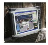
provides a good balance between performance and battery life. The aluminum-alloy body is very solid, sealed to IP54 specs, and can take a beating. Combined with full 1024 x 768 pixel XGA resolution on a 10.4-inch display with dual panel input, the MARS-3100R excels in applications that require as much screen real estate as possible in a very compact, rugged computer. [Read description and specs of the Advantech MARS-3100R]
