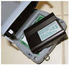
cases. They also pointed out that NiMH generally has better cold weather performance generally than Lithium Ion—a concern for a good number of Juniper Systems customers. Finally, they wanted to maintain consistency between the new Allegro MX and previous Allegro models. A change in battery technology would have meant a change in charging circuitry and maybe also a different case design, and that could have affected legacy peripherals and accessories.
