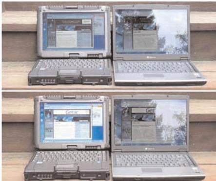
The V200 has a near perfect horizontal viewing angle but the vertical viewing angle is much narrower, and varying the vertical angle results in color shifts that can be distracting.
