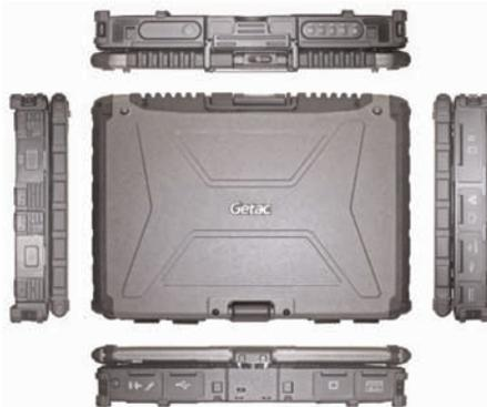
Getac also did a nice job protecting the V200's ports and connectors. Many rugged devices use one door to cover multiple ports. That makes no sense as you often need just one, so why expose the rest? The V200 has separate rubber/plastic covers for most ports. Each is clearly marked. Should one break or rip off, it is easily replaced.
