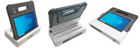
On the left is the office dock. It offers two extra USB 2.0 ports, an RJ45 LAN jack, and a 9-pin legacy RS232 serial port. The office dock includes a charging slot for an additional battery. On the right is the vehicle/wall dock. It provides the same extra ports, and has VESA 75mm and 100mm mounting screw hole cutouts in its back plate. Both docks are made of white plastic and powder-coated aluminium.
