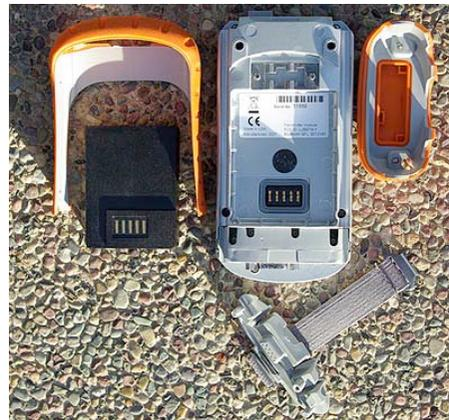
tic/rubber elastomer overmold by simply undoing a grand total of six screws and you find underneath an entirely more serious looking piece of equipment.
