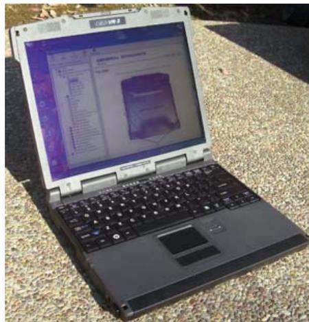
What DynaVue means is that you can be outdoors in the brightest sunshine and you can continue to work with the VR-2, even in direct sunlight. Some of the indoor vibrancy, of course, is gone, and the display takes on a greenish tint, but you can easily see it, and you can use it for work.
