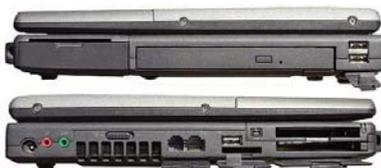
On the right side are the power jack, microphone and headphone jacks, wireless on/off, an RJ11 modem jack, a RJ45 gigabit LAN connector, a third USB 2.0 port, the multi-card reader, a mini-FireWire jack, and PC Card Type II and ExpressCard slots. The hard plastic protective doors are screwed onto the body of the computer for easy replacement.
