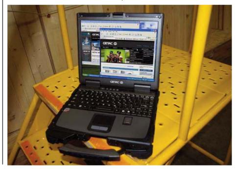
Getac chose a low-power processor that still offers good performance: the 1.6GHz Intel Core 2 Duo L7500 is the same chip Panasonic uses in the latest CF-30 (GD-Itronix uses a 1.83GHz Core Duo T2400 with a TDP of 31 watts).
