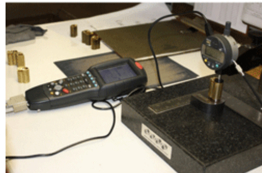
Datalogic Falcon connected to digital instrumentation for part inspection.
